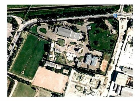
The pumps station was built in the period 1936-1944. Its present level of construction was achieved by the year 2011 via several former reconstructions. Until 1998, the pump station functioned as an end point pump station, and as of 1998 it forwards the water to be purified through a twin pressure pipe to the North-Pest Wastewater Treatment Plant.
